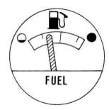
The fuel gauge pointer remains where it was even after key off, thus allowing operator or maintenance personnel to check the fuel level without much hassle.
